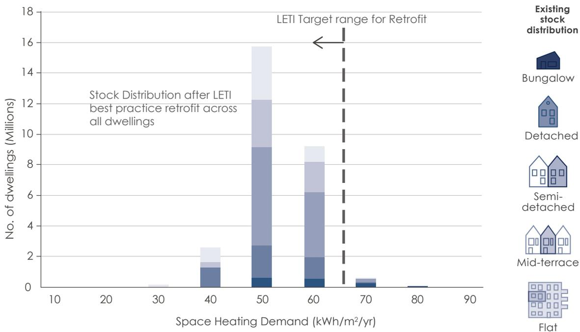
Figure 3.18 - UK Space heating demand distribution after 100% Best Practice Retrofit showing LETI's target range encompassing the vast majority of buildings.
