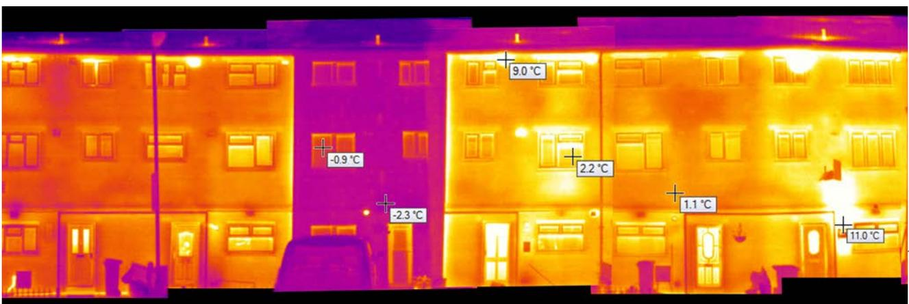
Figure 6.28 - Thermal imaging winter 2012 post retrofit, bere:architects
