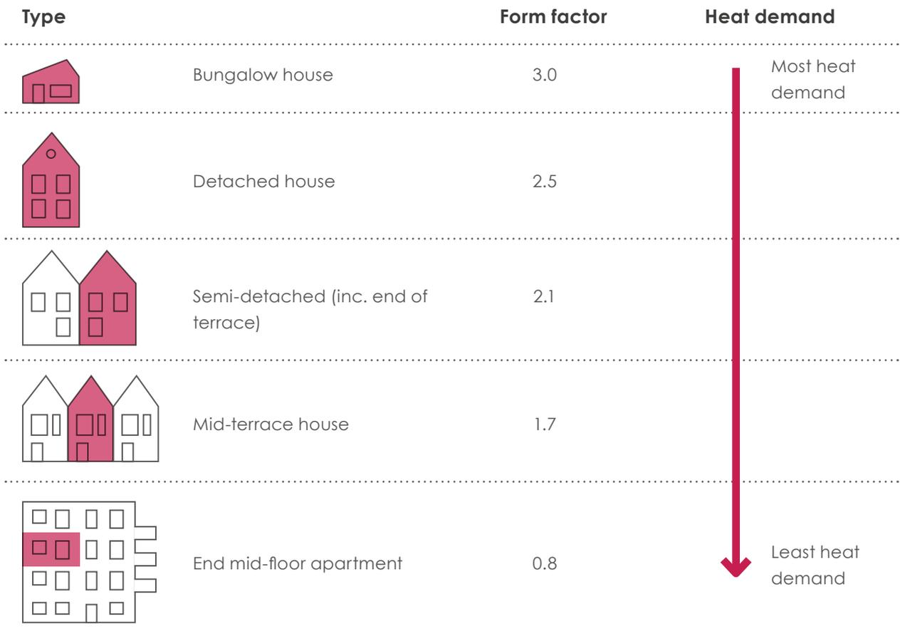
Figure 3.7 - The effect of lower (improved) form factors.
