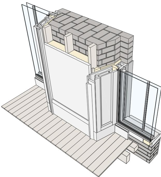
**Figure 6.30** - Axonometric showing insulation to walls, shutter box and secondary glazing to existing windows, Prewett Bizley Architects
