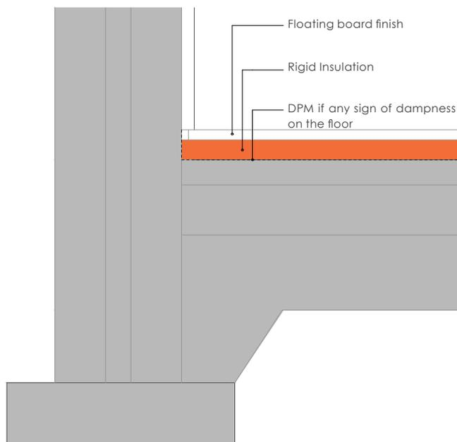
Figure C.6 - Insulation strategy for retained solid floor
