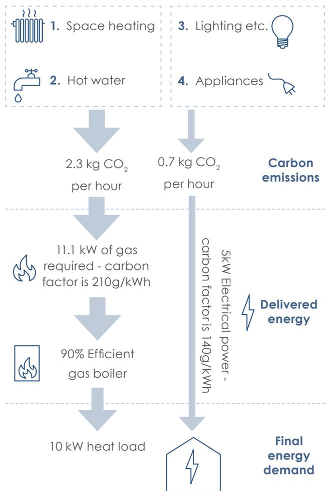
Figure A.3 - Average carbon Emissions associated with energy use
