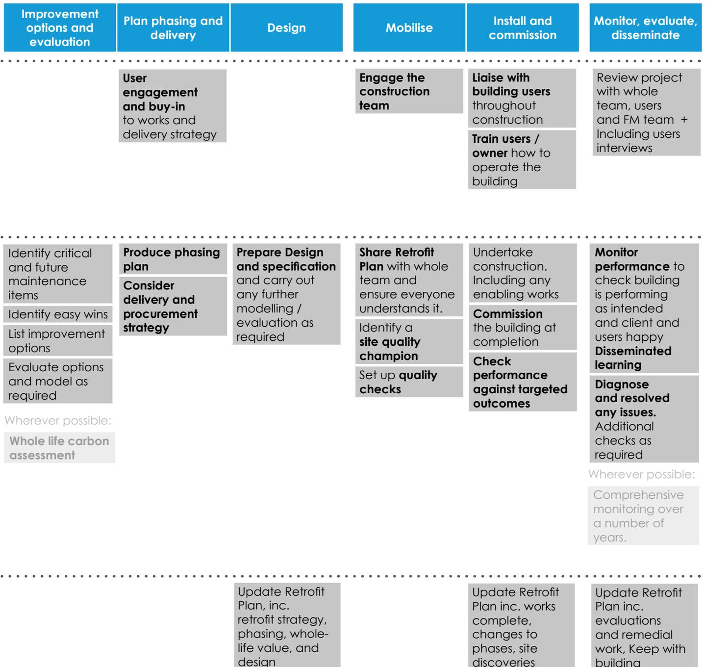
Figure 5.4 - LETI Retrofit Process flowchart mapped onto RIBA work stages
