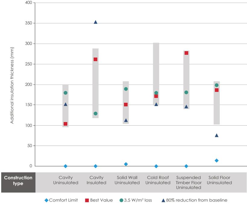
Figure G.4 - Thickness of additional insulation by baseline construction (ext temp 0 Degrees Celsius)
