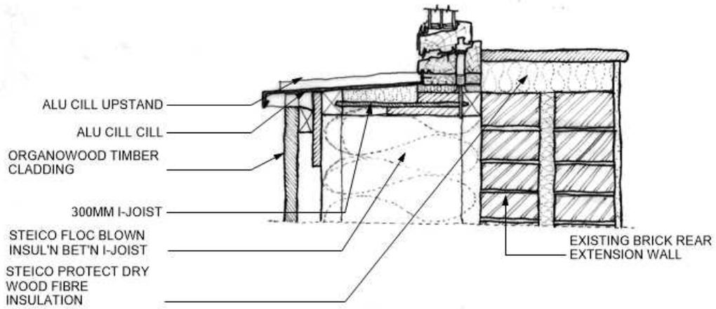
SECTION CILL DETAIL REAR ELEVATION
