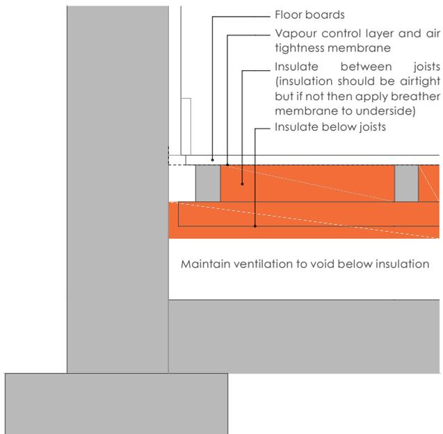
Figure C.5 - Insulation strategy for retained suspended timber floor
