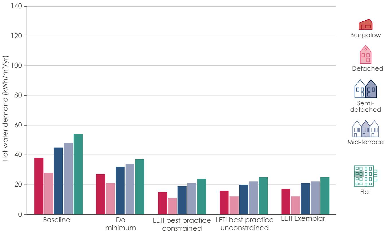
Figure 3.12 - Effect of varying retrofit scenarios on hot water demand, by building form.
