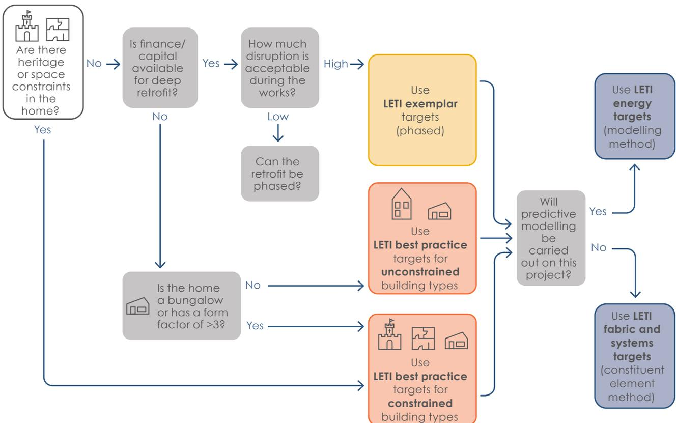
Figure 4.4 - Flowchart to assist target decision making
