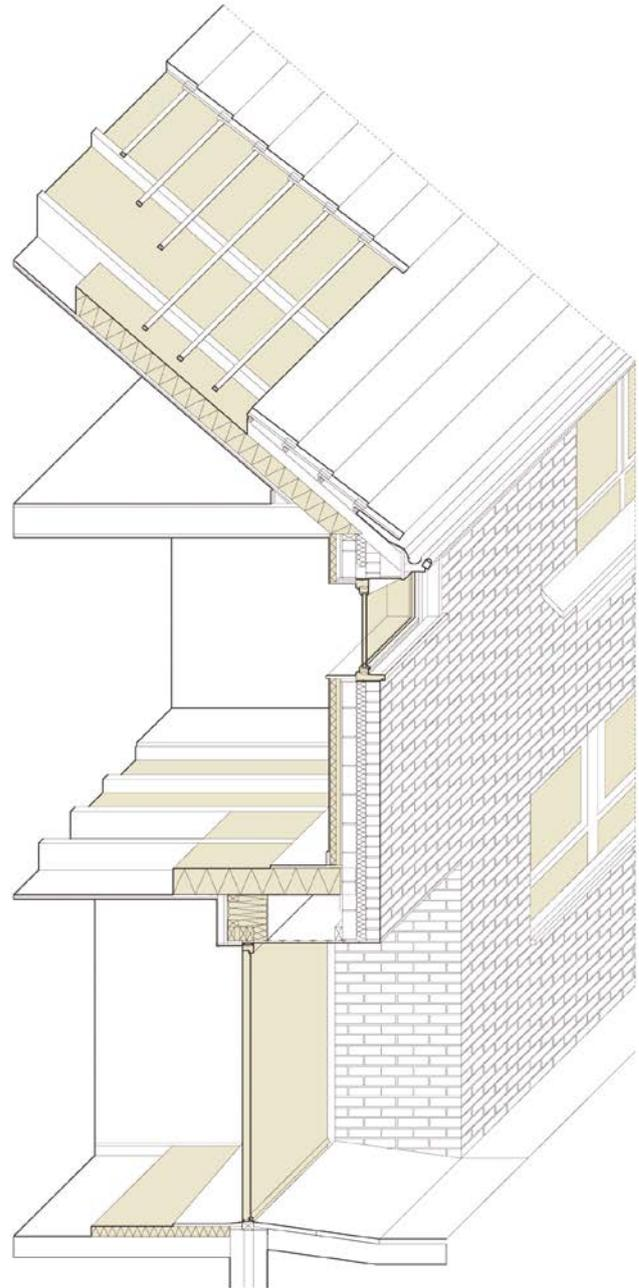
**Figure 6.4** - Detailed section post retrofit, from: Baeli, M., 2013, Residential Retrofit: Twenty Case Studies. RIBA Publishing, London<sup>6.1</sup>
