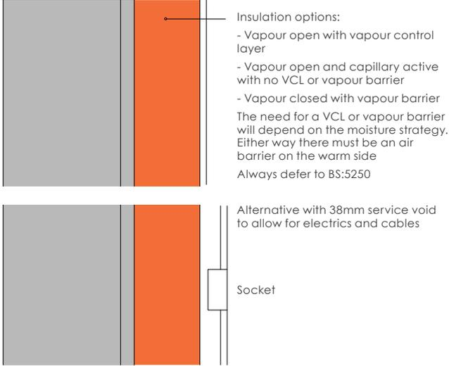
**Figure C.10**- Insulation strategy for solid wall - internal wall insulation (IWI)
