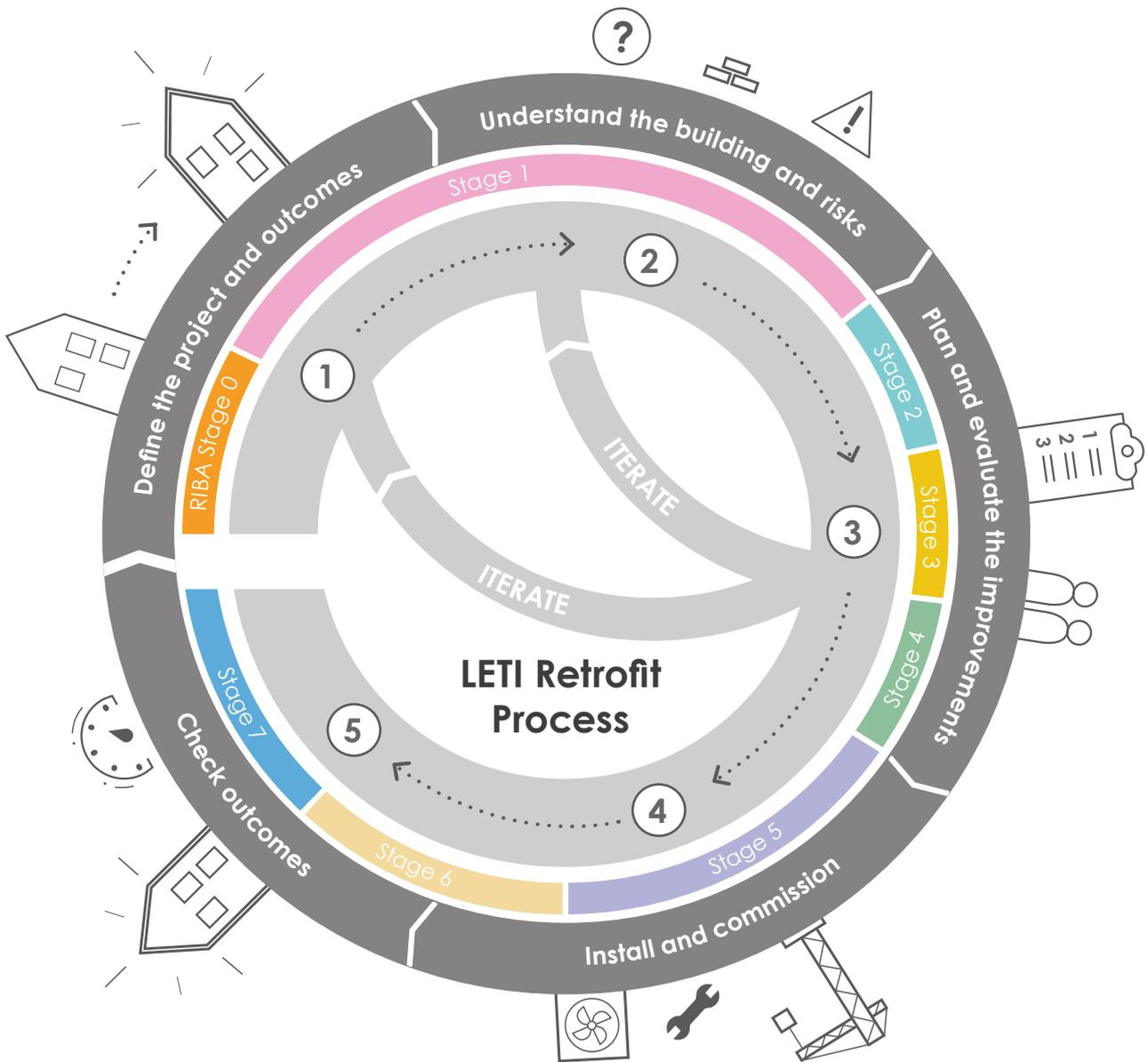
Figure 5.3 - LETI Retrofit Process summary diagram showing the key stages and how, where necessary, early design and evaluation gives a chance to revisit the project definition and building evaluation with new information.
