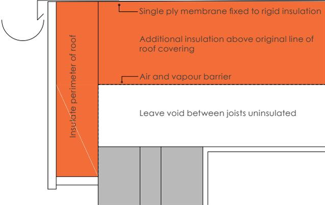
**Figure C.15**- Flat (warm) roof with additional insulation above roof line
