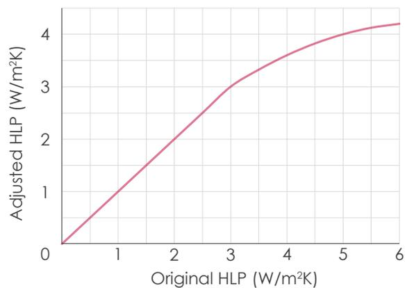
Figure E.5 - Heat Loss Parameter adjustment for cold dwellings
