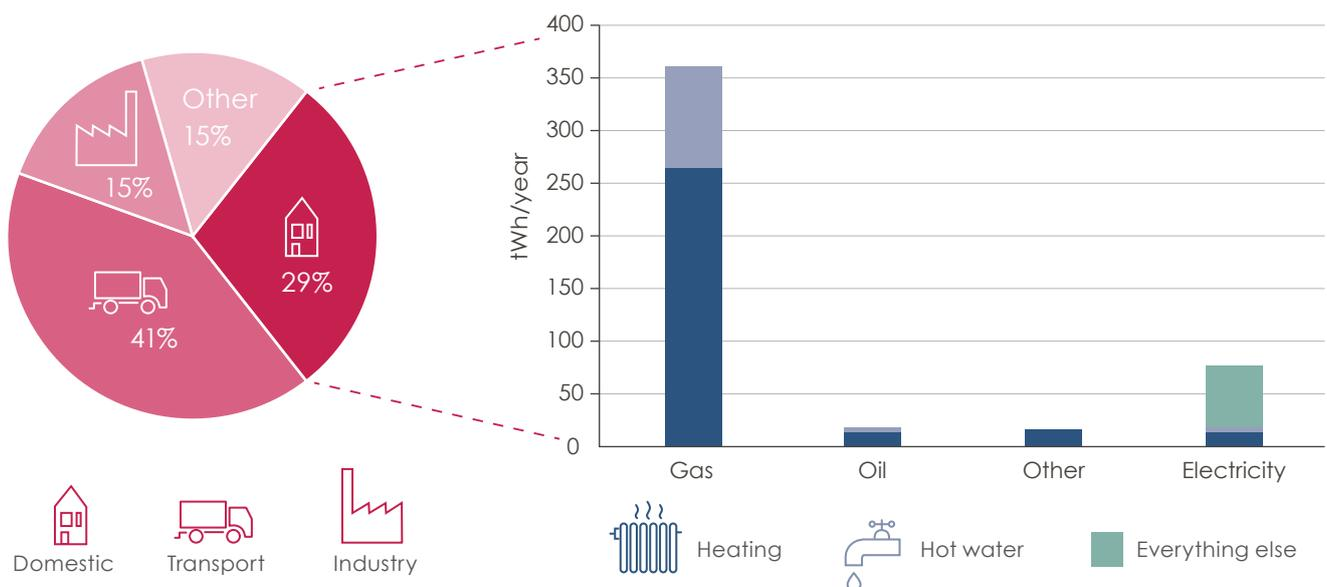
Figure 3.6 - UK sector consumption and domestic energy use breakdown (2018)<sup>3.3</sup>.
