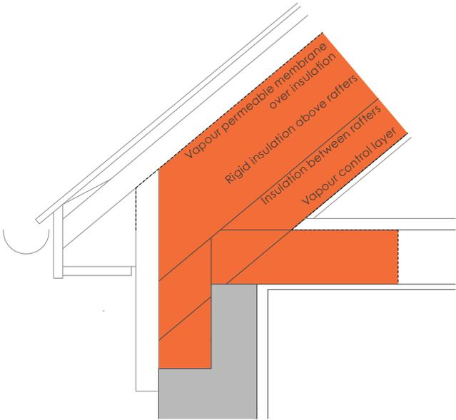
**Figure C.14** - Insulation strategy for cathedral roof with removed roof finishes, insulated between and below rafters, refinish roof ensuring ventilation above insulation
