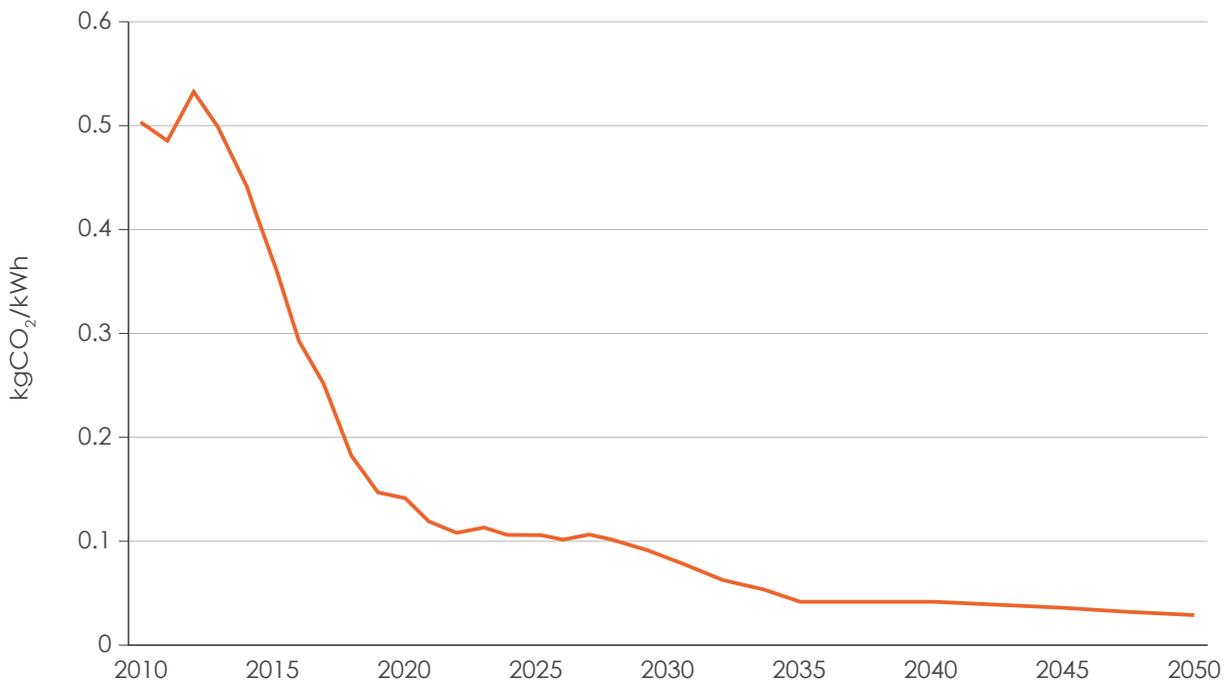
Figure 2.5 - Decarbonisation of the electricity grid.
